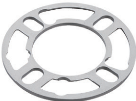
WS008 Description: 4/5Lug(100mm/4.25 to 120mm/4.75BC) 5mm/3/16"Thick
